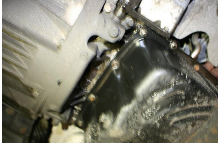
Photo no.4 confirms the rear section of the oil pan wet from oil.
