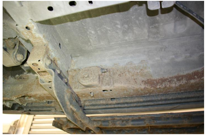
Photo no.8 is a view of the rear end chassis cross-member another common area for C.V.R.T. detection of corrosion.
