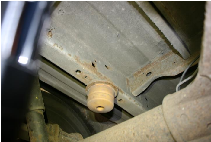
Photo no.5 is a common area for C.V.R.T. detection of corrosion on the O/S/R chassis bump stop area.
