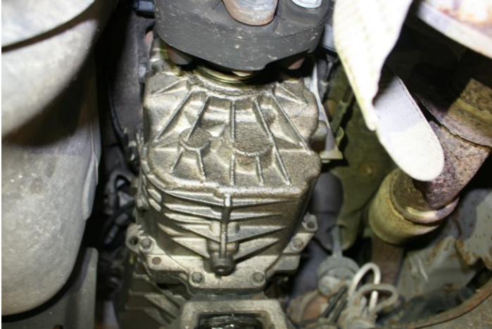
Photo no.3 is a view of the damp gearbox housing.
