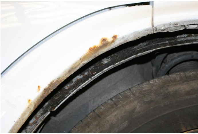
Photo no.7 is a view of the surface rust to the O/S/F wheel arch panel with oxidation of the panel evident.
